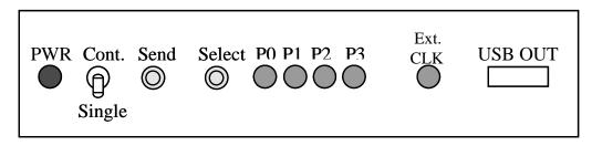
The front panel has one connector, six LEDs, and three switches:
